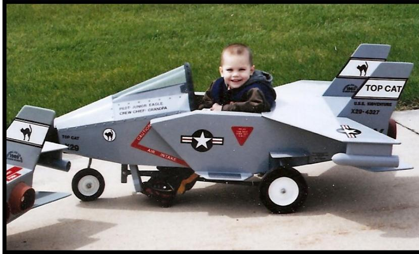
The TOP CAT is patterned after the F14 Tom Cat of Top Gun fame. The wing was swept back to act as an out-rigger. This model incorporates a unique nose wheel steering connected to the joystick. Fuselage and wings are constructed from 3/8” plywood. The windshild is made of a flexible material. Adjustable relay rods permit the pedal system to grow with the child. Top Cat’s decal set includes Air Force, Marine and Navy markings plus a full color instrument panel.
