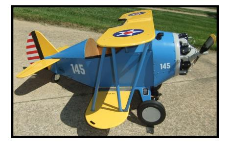
The Stearman was a very popular military trainer. The round engine, exposed cylinders give this toy distinct features. Fuselage and wings are constructed from 3/8" plywood and the engine case of 3/4" pine which is glued and turned to shape. The cylinders are made of pvc pipe. A adjustable pedal crankshaft assembly allows for a growing pilot and the joystick turns the plane by linkage to the tailwheel. The pedals also turn the prop assembly by use of a rubber drive belt.
